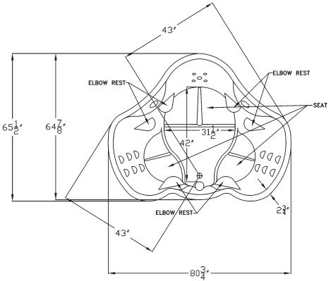
DIMENSION FROM FLOOR TO BOTTOM OF LIP - 23 3/4 DIMENSION FROM FLOOR TO TOP OF DECK - 28"
